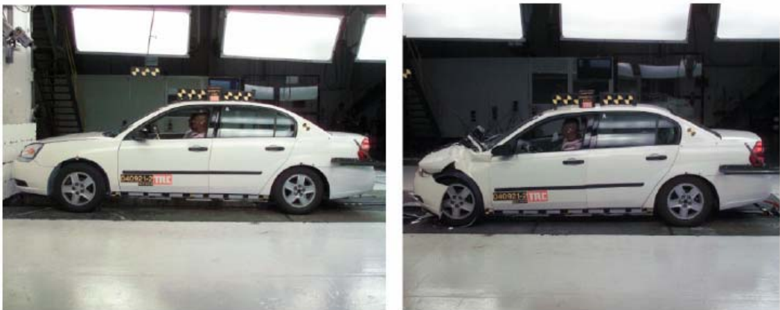
Fig. 3-41: NCAP 35 mph crash test [ASP06]
