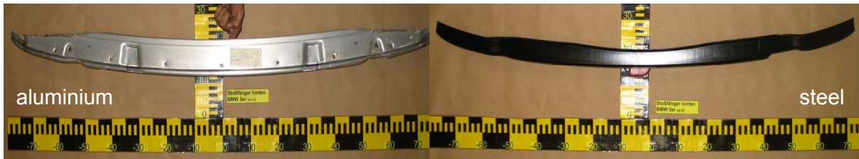
Fig. 3-36: Comparison of aluminium and steel rear bumper
