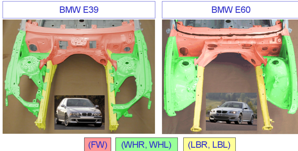
Fig. 3-38: Allocation of front structures
